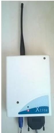
1. Identify that the red power light is on, this should be on constantly and identify that power is present.
